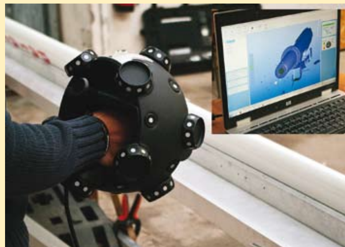
Scanning the mast with a laser scanner. Inset: A 3D-model of the mast being formed on the computer screen in real time. Photo: Paul Iatchkine, ENVSN.
